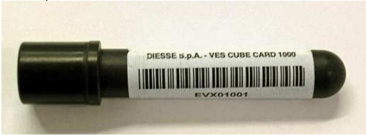
**fig. 3.3 a:** probeta “Check Device Transponder RF”
